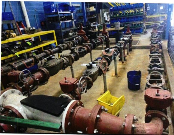
Veolia's NJ-Based Meter Test Bench Facility - For Meters 3-inch and larger
